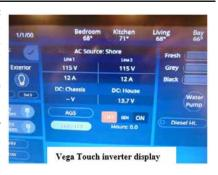
power. Refer to *Power Cut Out Switch* section for location of inverter disconnect switches. Inverter/charger 120-volt AC output is a pure sine wave type. The inverter/charger will operate most appliances, tools and other 120-volt AC equipment.
